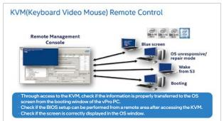
(e) Test result: The KVM session is connected from the manager PC to the vPro® PC, and the configuration can be modified in the BIOS screen of the vPro® PC on the KVM.
