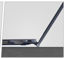
With ErgoLift hinge, the keyboard automatically tilts to the most comfortable typing positions.
