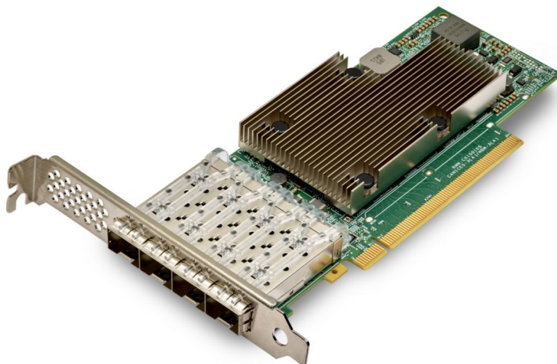
Figure 9. ThinkSystem Broadcom 57504 10/25GbE SFP28 4-Port PCIe Ethernet Adapter
