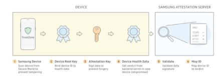
Because a <u>Samsung Attestation Key</u> (SAK) is unique to each device, it can tie data to a device through cryptographic signatures. The SAK signs the Attestation data to prove that it originated from the TrustZone Secure World on a Samsung Knox device.
