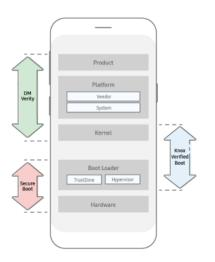
With KVB, component checks are conducted in the bootloader, and validations are made before system services are even started.
