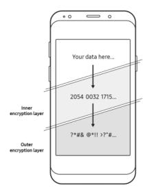
DualDAR's inner and outer security layers are independent and protect all information stored in the work profile when the device is in a powered off or unauthenticated state. Samsung Knox DualDAR leverages Android File Based Encryption (FBE) architecture.
