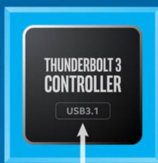
Integrated USB3.1 (10Gbps) host controller
