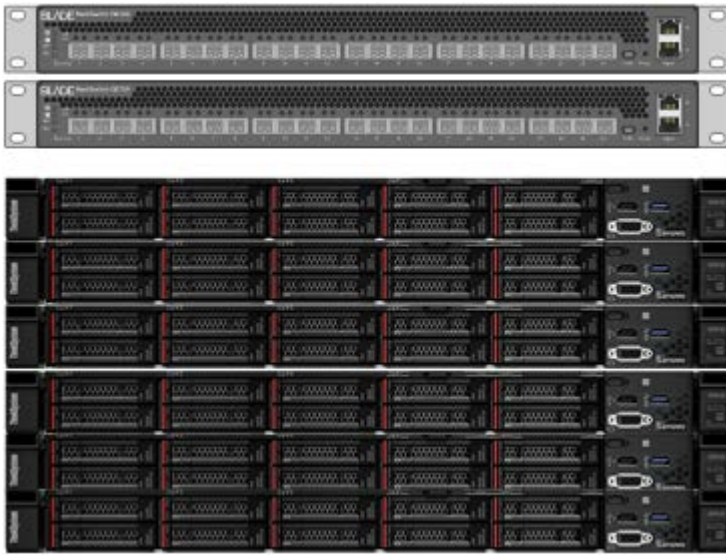
Figure 8: Deployment configuration for 1200 dedicated users using vSAN on ThinkSystem servers
