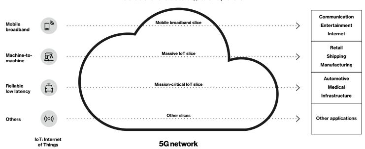
Figure 2: 5G network slicing (source: sdxcentral4)
