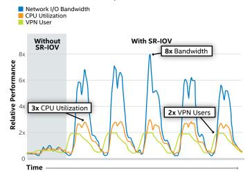
Figure 3. Intel IT testing of on-premises virtual VPN gateway systems show clear benefits from SR-IOV enablement. Note that we capped the gateway at 25 percent CPU utilization for load distribution across multiple gateways.
