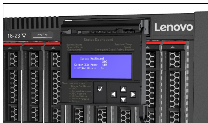
Figure 15. Integrated diagnostics panel with LCD display
